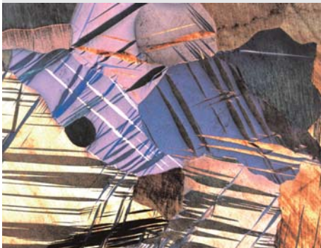
Cast tin with deformation twins, 200 x
